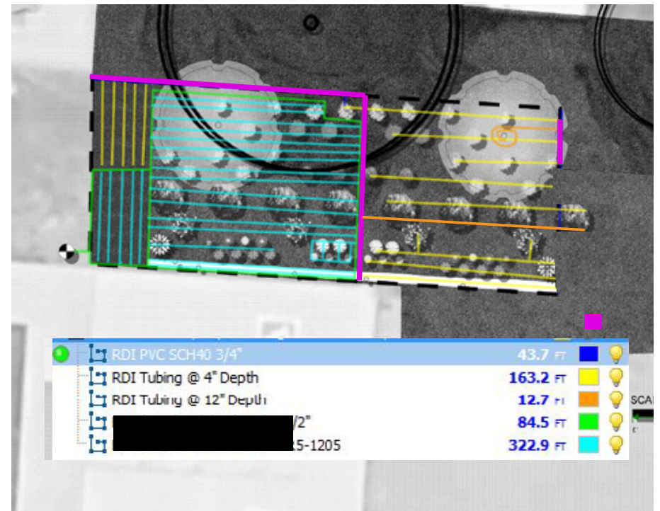
Irrigation design: GrowStream™ vs. leading subsurface drip. GrowStream™ shows simplicity in layout, flexibility in design, and reduced installation labor. Standard drip requires twice as much product to meet the varying plant water requirements.
